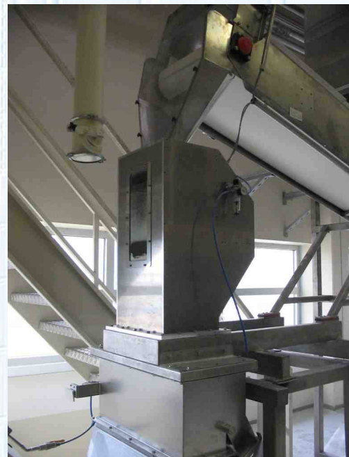
FlowSlide installation behind a conveyor belt.
